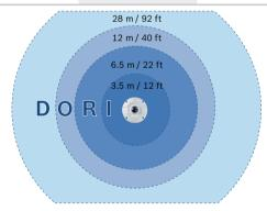
When mounted at a height of 3 m (10 ft) the 360° version of the camera has the following coverage radius for the four levels:
